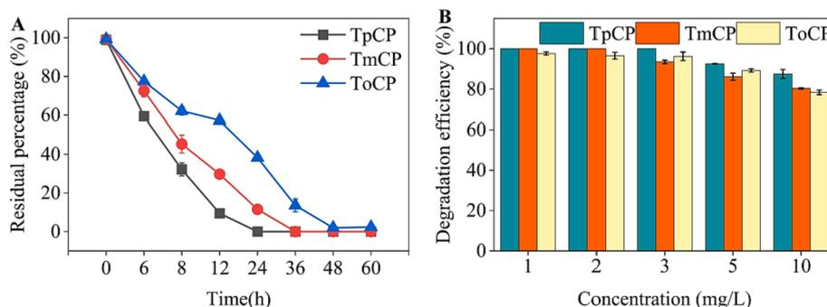
Fig. 4. Effects of contact time (A) and initial concentration (B) on TpCP, TmCP, and ToCP biodegradation by microbial consortium GY.
