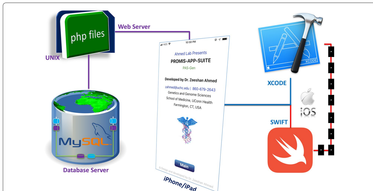
Fig. 2 PAS-Gen components design, development, and data flow. PAS-Gen is an iOS app developed with Swift programming language, XCODE integrated development environment for MacOS, MySQL database management system, PHP scripting language, and UNIX-based web and database servers
